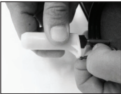
11. Slide cylinder onto piston and attach to pump piston rod.
