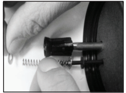
9. Install new rod gasket (161013), first rod washer (161065), rod spring (161014), then second rod washer (161065).
